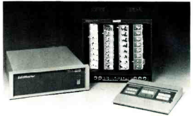
The Asaca editing previewer allows the display of video frames.
