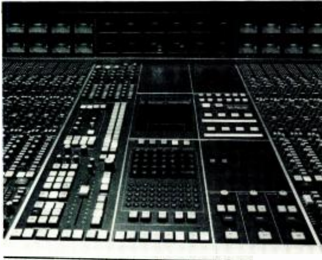
Solid State Logic's 6500E automated mixing console.
