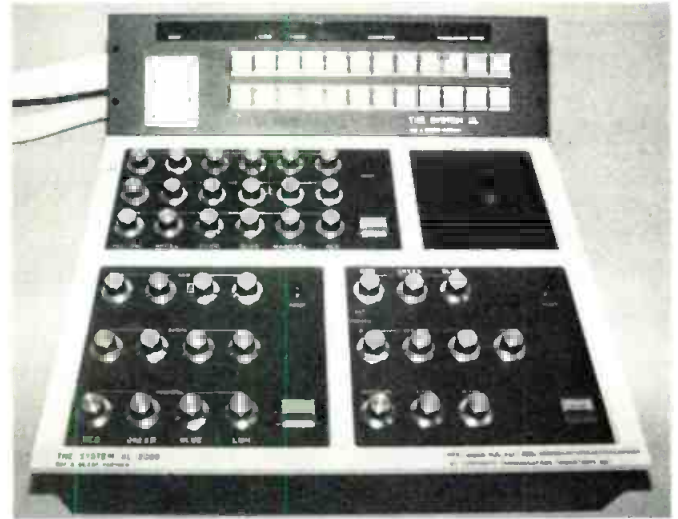
Corporate Communications' System 2000 scene-by-scene color corrector.
